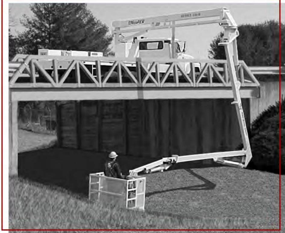
and a 6' long 4th boom pickup allowing placement of workers behind girders. The reach of the Snooper Series 230 from the second turret to end of the basket is 34' - 5/8". A spacious 60" long x 36" wide x 42" high basket and proportional hydraulic controls are standard features as well.
