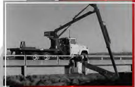
**Designed for handling and placing conduit and pipe under or along side a bridge structure.**
